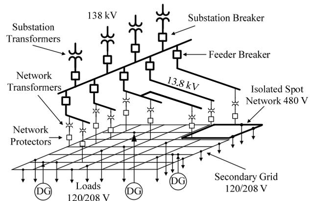
Fig. 1. Illustration of a LV secondary network including: high voltage, substation, loads, transformers, DG, and a typical structure of an isolated spot network. In NYC the low voltage networks operate at 208/120 V and isolated spot networks are fed at 460 V.
