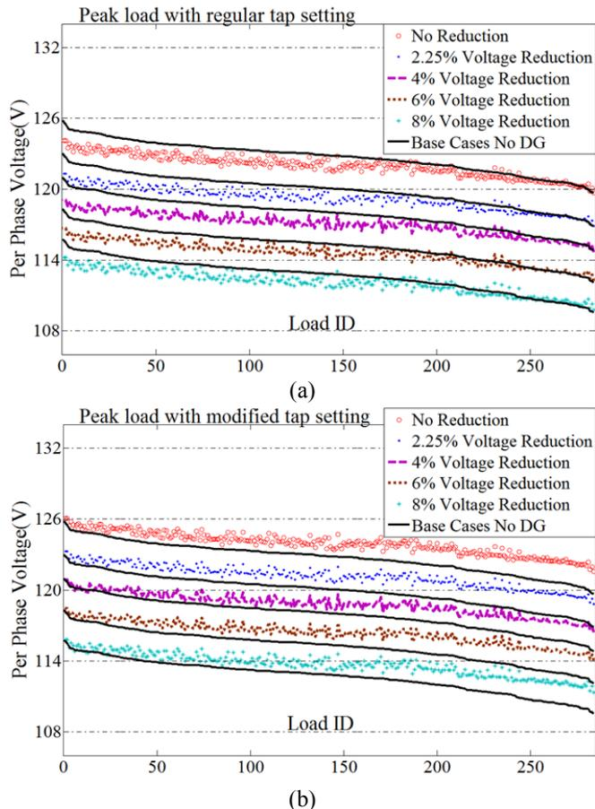
Fig. 8. Sutton network voltage profile for customers at 120 V during peak load hour; (a) regular tap setting; (b) modified tap setting. Results for base case and CVR with no DG penetration are in solid lines.
