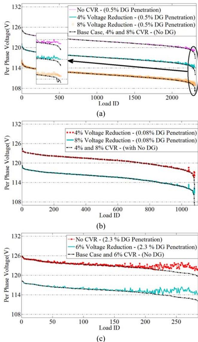
Fig. 7 Comparison of voltage profile for loads at 120 V without DG penetration (dash dotted lines) and with DG penetration. Results are shown for the base case with no voltage reduction, 4% and 8% CVR; (a) for Yorkville; (b) Madison Square; (c) Sutton with no voltage reduction and 6% CVR.
