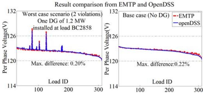
Fig. 2 Comparison of results for customer voltage profile at 120 V from OpenDSS and EMTP for the worst case scenario (left) and base case with no DG (right) reported in [16].
