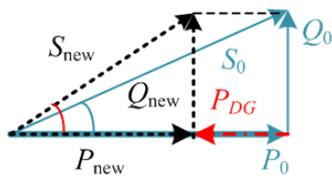
Fig. 9. Illustration of the network power triangle with no DG penetration (solid lines), total power supplied by all DGs (dash-dotted line), and the new network power triangle DG penetration (dashed lines).
