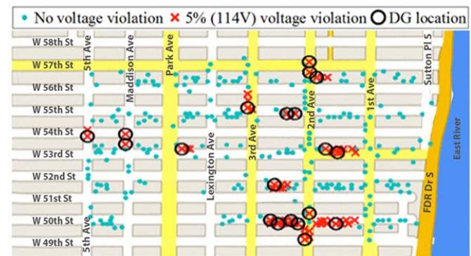
Fig. 6. Geographical voltage distribution in Sutton network for 6% voltage reduction of the peak hour of the year with 62 voltage violations detected of over 5% (under 114 V). Twenty nine localized DG allocated on structure points under voltage violation. Underlying map ©2014 by Google.
